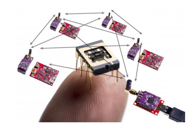
NO<sub>2</sub> sensor + network hardware for wireless sensor network
