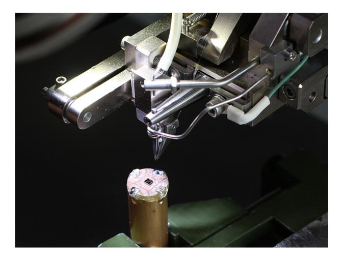
Wiring of a sample for magnetoresistance measurements. Credit: Avci, Mendil and Gambardella / ETH Zurich
