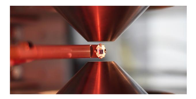
A sample between the poles of an electromagnet. Credit: Avci, Mendil and Gambardella / ETH Zurich
