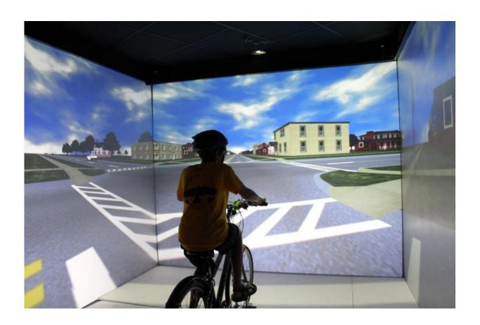
The University of Iowa's Hank Virtual Environments Lab allows researchers to safely study the factors that put kids at risk when they're biking or walking across the street. Credit: Hank Virtual Environments Laboratory at the University of Iowa
