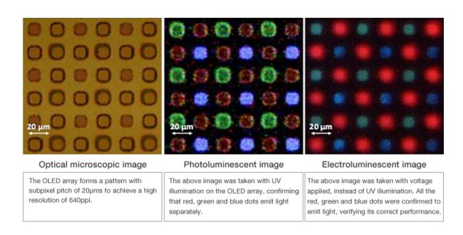
Fujifilm Corporation and nano-electronics research institute imec have demonstrated full-color organic light-emitting diodes (OLED) by using their jointly-developed photoresist technology for organic semiconductors, a technology that enables submicron patterning. This breakthrough result paves the way to producing high-resolution and large organic Electroluminescent(EL) displays and establishing cost-
