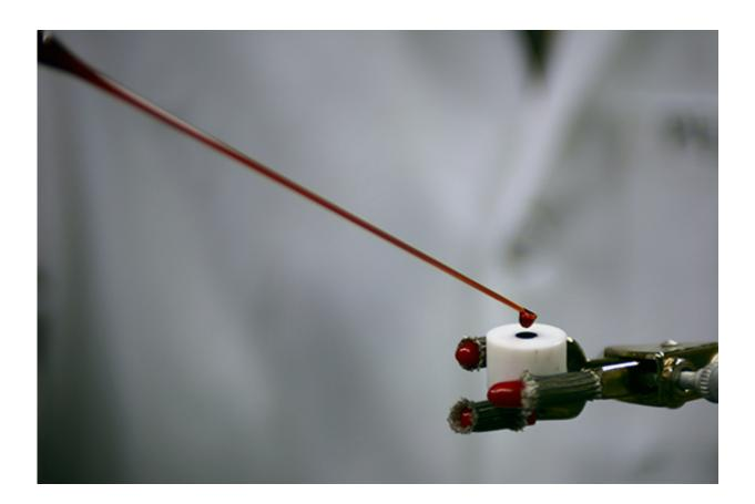
Drop casting a catalyst slurry onto an electrode results in thin layers ready for electrochemical tests.
