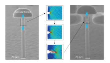
Experimental measurements (left and right) and molecular dynamics simulations (middle) of metallic glass nanopillars reveal that structural flaws play important roles in determining material strength. Credit: American Chemical Society
