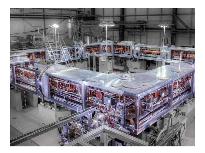
The CRS storage ring at the Max Planck Institute for Nuclear Physics shortly before cooling down: In this unique instrument, molecular ions are cooled to minus 263 degrees Celsius and sent onto a 35.4-metre long orbit at an extremely low pressure in order to investigate astrochemical processes and their quantum
