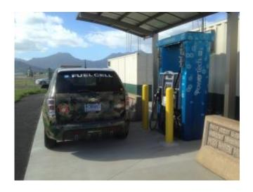
Electric vehicles fuel up with hydrogen at Marine Corps Base Hawaii. Credit: Mitch Ewan, HNEI
