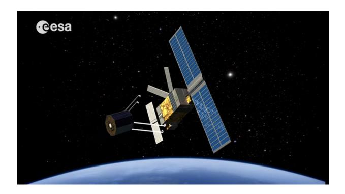
Simulations of orbital debris show that actively removing large items of debris, such as entire derelict satellites, should help to stabilise the population and prevent cascading collisions. ESA has performed a system study for an Active Debris Removal mission called e.Deorbit. Credit: ESA
