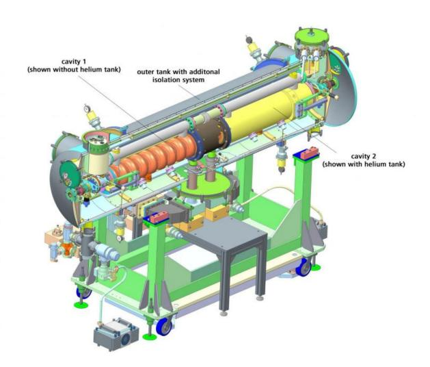
Cross-section through the highly complex accelerator module with its thermalinsulation system and the superconducting resonators (cavities). Credit: Helmholtz-Zentrum Dresden-Rossendorf (HZDR)
