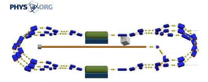
Schematics of the MESA accelerator. The green cylinders represent the two accelerator modules. After two full rounds of recirculation, the electron beam reaches an energy of 150 MeV. Credit: Institute of Nuclear Physics, JGU
