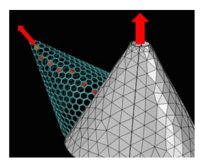
Flexing graphene may be the most basic way to control its electrical properties, according to calculations by theoretical physicists at Rice University and in Russia.
