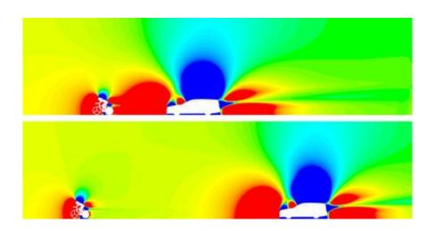
Images of the computer simulations. The top image shows what happens when a team car follows at 5 meters, the bottom image shows a distance of 10 meters. Clearly visible is how at a shorter distance the red area in front of the team car overlaps with the turbulent - and slowing - wind flows behind the rider. Credit: TU Eindhoven
