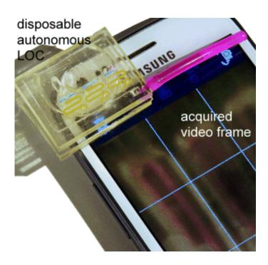
There is growing demand for point-of-care diagnosis worldwide using low-cost, autonomous, and disposable devices. Scientists in Sweden have developed a disposable lab-on-a-chip unit that is manufactured by 3D printing technique and equipped with an integrated 3D-printed optical lens system which serves as an interface for direct readout by any regular cell phone camera. As the scientists report in the journal *Angewandte Chemie*, their device reliably performs quantitative chemical sensing, and
