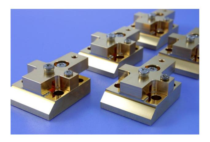
Laser bars with optimized mounting for high-power operation on CCP mount, developed within the CryoLaser project. Credit: FBH/P. Immerz
