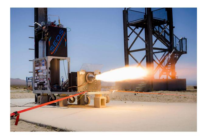
UC San Diego Chapter of Students for the Exploration and Development of Space were able to successfully test the latest version of their 3-D-printed rocket engine. Credit: Erik Jepson/UC San Diego
