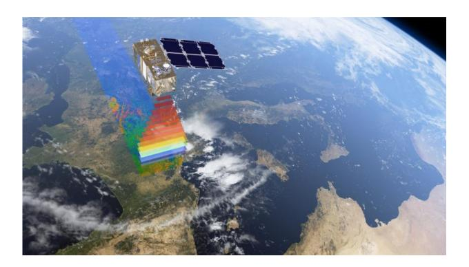
Combining high-resolution and novel multispectral capabilities, a swath width of 290 km and frequent revisit times, the new Sentinel-2 mission offers views of Earth's changing lands in unprecedented detail. Credit: ESA/ATG medialab
