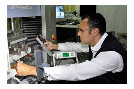
Dr. Sahmaran tests the performance of healed ECC specimen under mechanical loading
