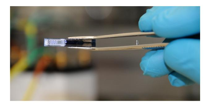
ETH researchers' miniature CO2 sensor is pictured: chip with a thin layer of the polymer-nanoparticle composite. Credit: Fabio Bergamin / ETH Zurich
