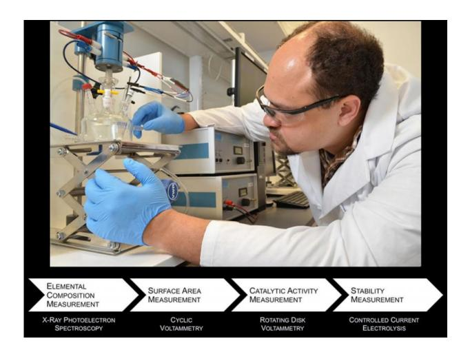
Dr. Charles McCrory is setting up a rotating disk electrode experiment, which is used to measure a material's catalytic activity and stability under conditions that are required for a working water-splitting device. These measurements follow a separate procedure in which the sample's surface composition is characterized by
