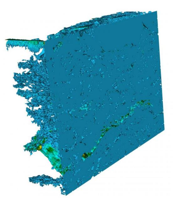
Simulation of resolved steady-state flow in fractured Marcellus shale based upon FIB-SEM imagery obtained by Lisa Chan at Tescan USA, processed by Terry Ligocki (Berkeley Lab). Credit: Tim Kneafsey (Berkeley Lab)
