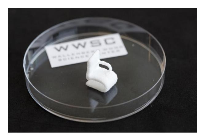
The tiny chair made of cellulose is a demonstrational object printed using the 3-D bioprinter at Chalmers University of Technology. Credit: Peter Widing
