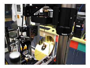
A sapphire rod being melted in the Laser Heated Pedestal Growth system. A sapphire seed crystal is being lowered onto the molten sapphire rod to begin the growth of a single-crystal sapphire fiber.
