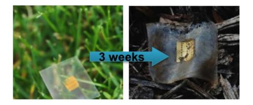
A fresh CNF based microwave silicon transistor chip. After three weeks of putting it in a woodpile, the chip was partially degraded with the help of fungi. Credit: Jung-Hun Seo, Shaoqin Gong and Zhenqiang Ma/University of Wisconsin-Madison
