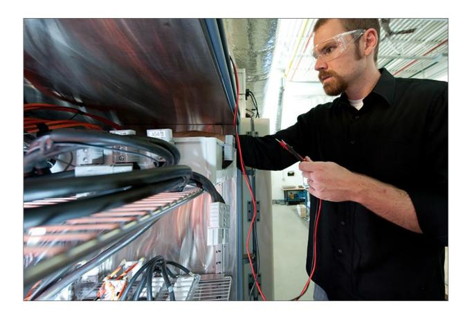
NREL's Jeremy Neubauer measures battery voltage in an environmental chamber at the Thermal Test Facility. NREL is identifying battery second use (B2U) strategies capable of offsetting vehicle expenses while improving utility grid stability. Credit: Dennis Schroeder
