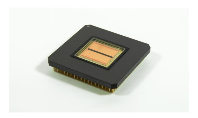
This 60-line sensor is twice as fast as previous systems. Credit: Fraunhofer IMS
