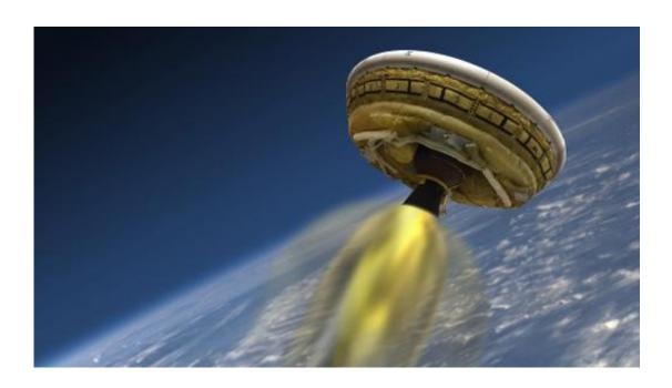
A NASA artist's concept shows the test vehicle for NASA's Low-Density Supersonic Decelerator(LDSD), or flying saucer, designed to test landing technologies for future Mars missions
