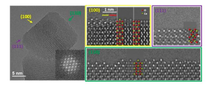
The image on the left shows the general shape of a cubic CeO2 nanoparticle. The images on the right show edge-on views of three exposed surfaces at atomic resolution. The atomic models are overlaid on the simulated images to illustrate atom positions. Credit: Northwestern University
