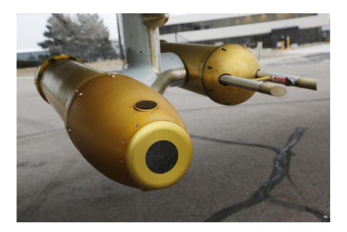
The Differential Optical Absorption Spectroscopy instrument hangs under the wing of a research aircraft. Relying on measurements from the instrument, CIRES Fellow Rainer Volkhamer and international colleagues report that halogens, natural chemicals from the ocean, can contribute to much more vigorous atmospheric chemistry than previously understood. The discovery may help explain levels of mercury contamination in the air, on land and in the
