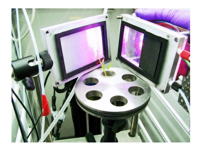
A radio tracer chamber at Brookhaven National Laboratory was needed to test if *Setaria viridis* actually used nitrogen produced by the bacteria. The scientists allowed only one leaf to contact the radioactive nitrogen, so they could truly tell if it was being used. Credit: Fernanda Amaral
