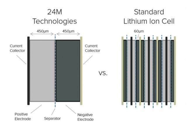
Cross-sectional diagram shows how the new design for lithium-ion battery cells by 24M increases the thickness of electrode layers and greatly reduces the number of layers needed, reducing manufacturing costs. Credit: 24M
