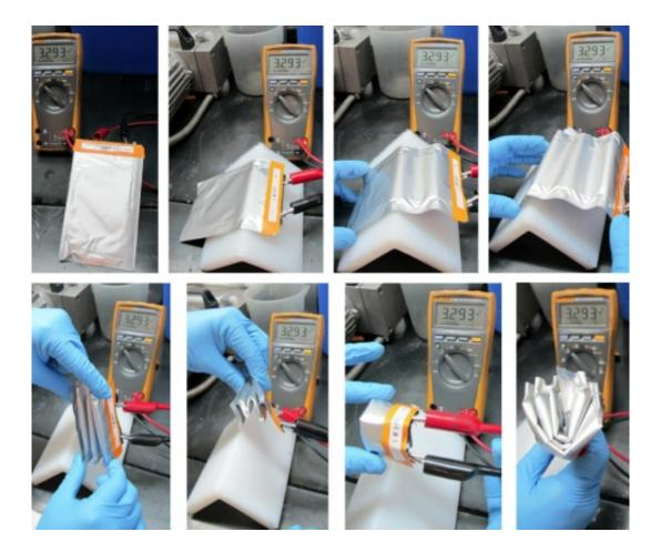
Unlike conventional, solid lithium-ion batteries, the new semisolid cells are flexible enough to be bent and folded multiple times without affecting their performance, as shown by the constant voltage readings in this test. Credit: 24M
