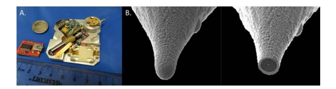
A. The new patent includes a compact programmable NANOrotator that allows the fabrication of "smart" tips. B. Coaxial "smart" tips serve as novel x-ray detectors, shown before (left) and after (right) nanofabrication. Credit: Argonne National Laboratory
