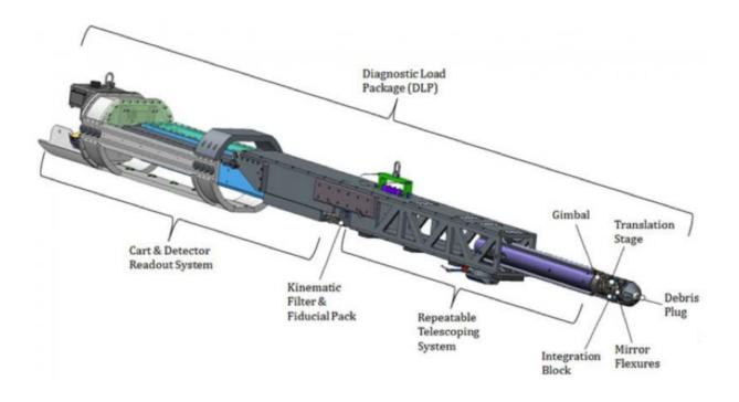
The KBO X-ray microscope diagnostic load package for use in a NIF diagnostic insertion manipulator.
