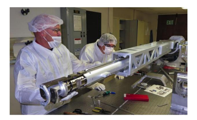
Diagnostic technician Jesse Hamblen (left) and system manager Jay Ayers mount the Kirkpatrick-Baez optic (KBO) telescoping snout on its carriage rails. The KBO will provide improved resolution (better than 10 microns) and 4.5 times greater collection angle compared to a pinhole imaging system. Credit: James Pryatel/LLNL
