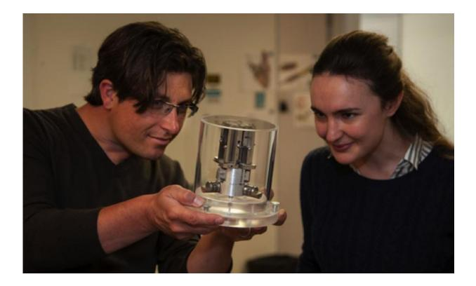
The KBO X-ray microscope diagnostic load package for use in a NIF diagnostic insertion manipulator. Jay Ayers and Louisa Pickworth examine a mirror pack for the KBO diagnostic. Credit: James Pryatel/LLNL
