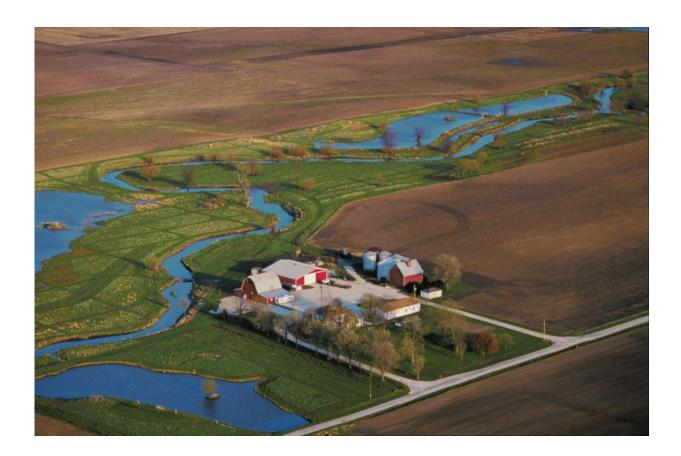
A spring view of wetlands along the Embarras River in southern Champaign County. The wetlands were constructed and first studied for nitrate runoff from 1994-98. Results from recently conducted research on the same wetlands show an overall 62 percent nitrate removal rate and little emission of nitrous oxide, a potent greenhouse gas. Credit: University of Illinois
