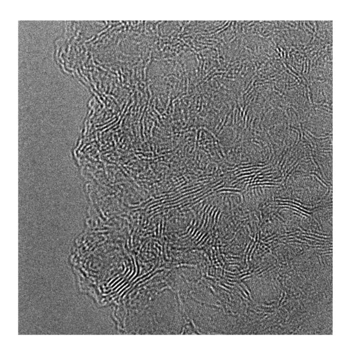
An electron microscope image shows the edges of graphene flakes burned into a
