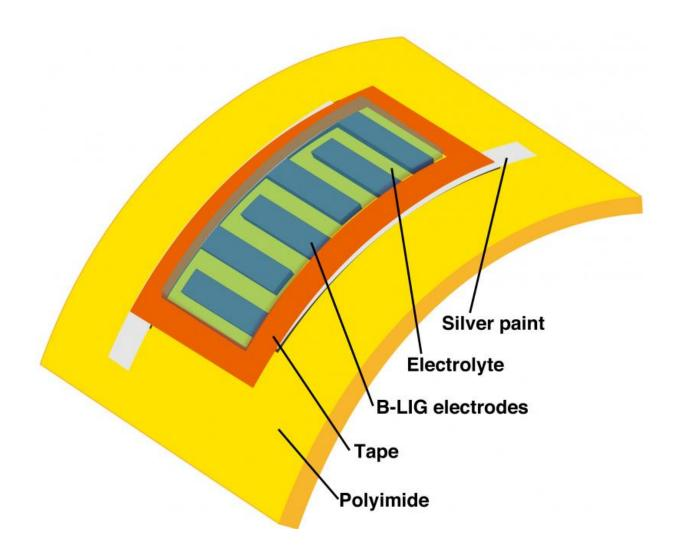
A microsupercapacitor designed by scientists at Rice University may find its way into personal and even wearable electronics. The lab upgraded its laser-induced graphene device by treating the raw polymer material in advance with boron. Credit: Tour Group/Rice University
