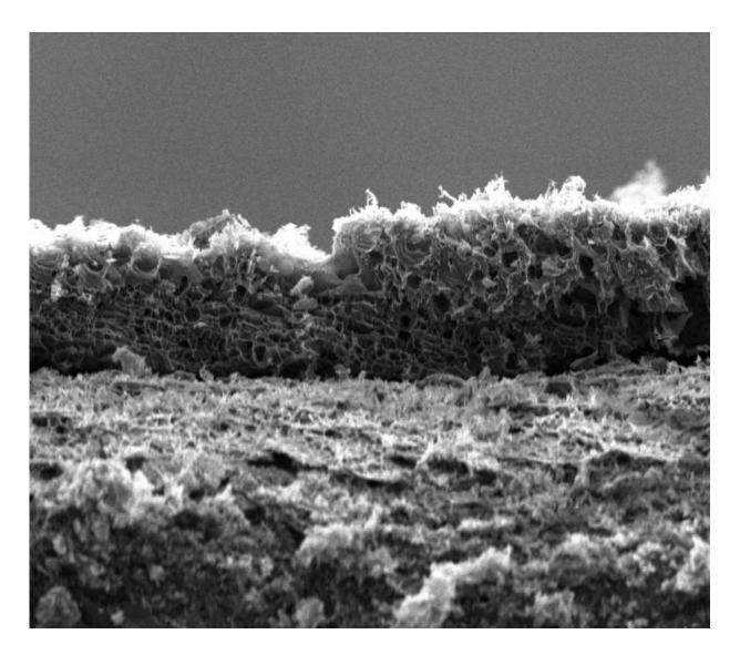
An electron microscope image shows the foamy surface of a polyimide treated with boron and burned with a laser to create a lattice of graphene flakes. The material shows promise as a highly efficient, flexible energy storage device for electronics. Credit: Tour Group/Rice University
