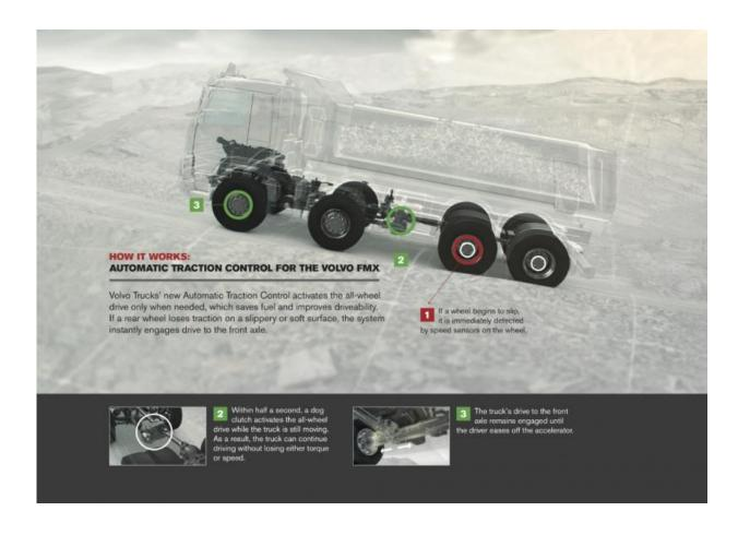
Volvo Trucks' new feature Automatic Traction Control activates the
