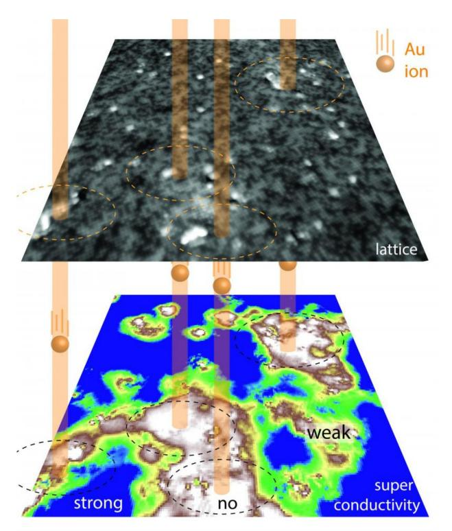
High-energy gold ions impact the crystal surface from above at the sites indicated schematically by dashed circles. Measurement of the strength of superconductivity in this same field of view, as shown on the lower panel,
