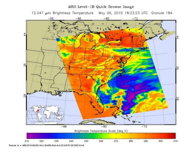
On May 06, the AIRS instrument aboard NASA's Aqua satellite saw cloud top temperatures as cold as 210 kelvin/-63.1F/-81.6C (purple) in powerful thunderstorms within Tropical Disturbance 90L. Credit: NASA JPL/Ed Olsen
