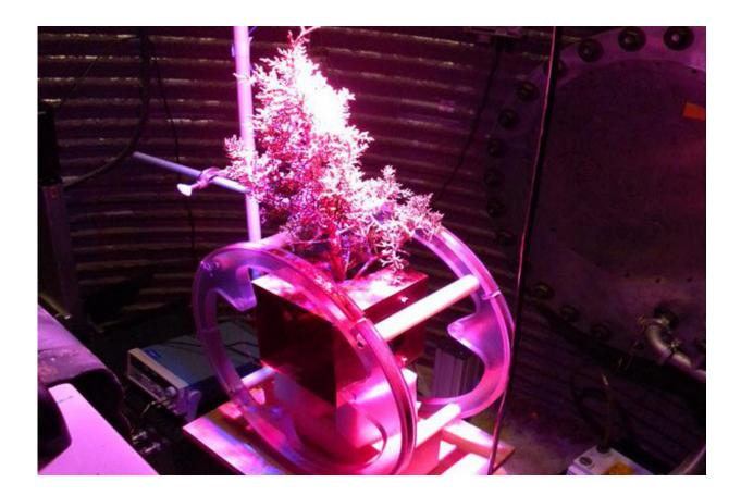
Photograph of the ULF-NMR and neutron imaging experiment: the experiment is conducted under a special growth lamp to induce stomatal opening. An LED lamp (no magnetic noise and heat produced) provides a high density of photosynthetically active radiation. To human eyes it looks pinkish because the wavelength band starts at 400nm and it cuts out some of the blues.
