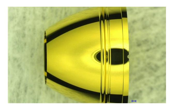
Rugby hohlraums resemble a cylinder, with the corners of the can rounded off to minimize surface area. The major sink of energy in a hohlraum is through the wall surface area, and the rugby shape helps to appreciably reduce this energy loss. Half of the hohlraum is shown here.
