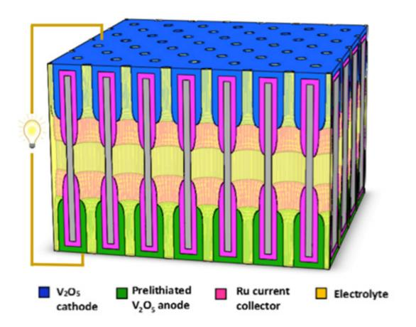
Complete nanobatteries are formed in each nanopore of a dense nanopore array (2 billion per square centimeter), using atomic layer deposition to carefully control thickness and length of multilayer concentric nanotubes, which serve as electrodes at each end.
