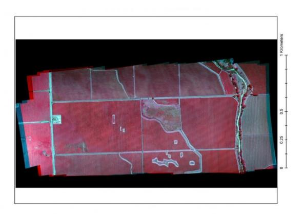
More data means more efficient water use. Different spectral band images, like this false-color infrared view of a field, can be combined to provide highresolution information about surface temperature, water use, plant nutritional
