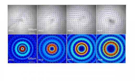
Microparticles are twisting in an acoustic vortex. Top row shows the experimental observations (0.5 micron particles) and the bottom row the predicted acoustic energy distribution. Credit: University of Bristol
