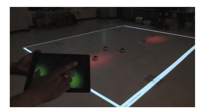
A human operator can touch the screen in multiple locations to control the light and the robots. Credit: Georgia Tech
