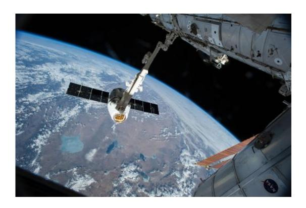
This NASA image taken April 17, 2015 shows the Canadarm 2 reaching out to grapple the SpaceX Dragon cargo spacecraft and prepare it to be pulled into its port on the International Space Station
