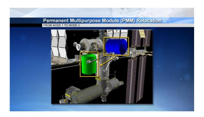
This illustration shows the current location (blue) of the Permanent Multipurpose Module (PMM) on the International Space Station and the location to which it will be repositioned (green) during the May 27 move. Credit: NASA
