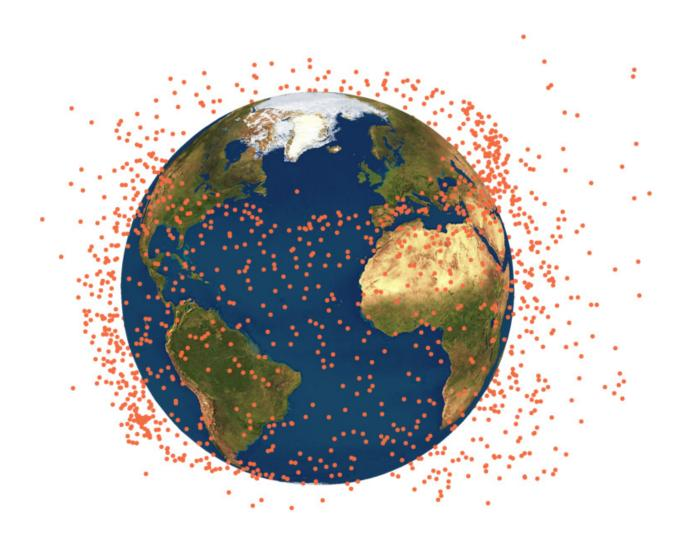
The spreading of the fragmentation cloud to form a band of debris (exaggerated size).
