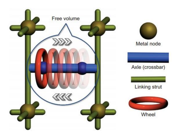
MOF materials are commonly constructed from a combination of rigid linking struts (green) and metal nodes (brown). Credit: Kelong Zhu et al. *Nature Chemistry*, 2015: doi:10.1038/nchem.2258
