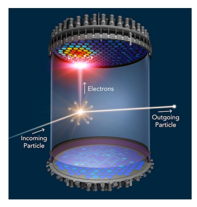
When a WIMP – a hypothetical dark matter particle – collides with a xenon atom, the xenon atom emits a flash of light (gold) and electrons. The flash of light is detected at the top and bottom of the liquid xenon chamber. An electric field pushes the electrons to the top of the chamber, where they generate a second flash of light (red). LZ will be searching for a particular sequence of flashes that cannot be due to anything other than WIMPs. Credit: SLAC National Accelerator Laboratory
