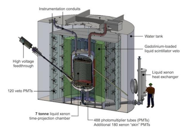
In addition to the shielding provided by its location one mile underground, LZ's xenon vessel will be surrounded by several layers of detectors and shielding that help suppress unwanted signals from particles other than WIMPs. Credit: LZ collaboration
