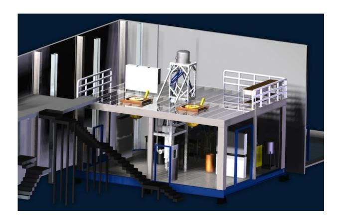
SLAC is setting up a platform for testing a prototype detector where members of the LZ collaboration will perform a variety of system tests. SLAC is also building a xenon purification plant. Credit: SLAC National Accelerator Laboratory
