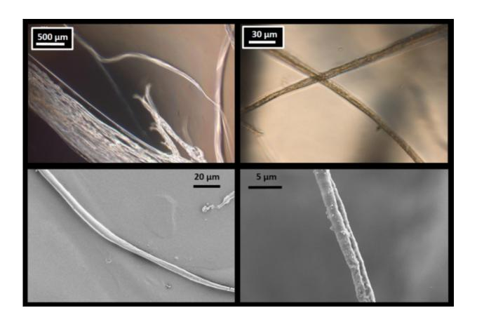
Microscope images of lab-produced fibers confirm the results of the MIT researchers' simulations of spider silk. At top are optical microscope images, and, at bottom, are scanning electron microscope images. At left are fibers 8 micrometers across, and, at right, are thinner, 3 micrometer fibers.
