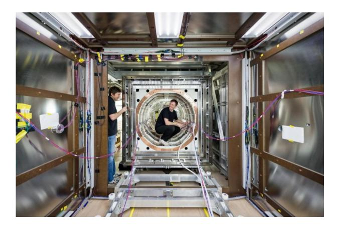
An international team of physicists has developed a shielding that dampens low frequency magnetic fields more than a million-fold. Using this mechanism, they have created a space that boasts the weakest magnetic field of our solar system. The physicists now intend to carry out precision experiments there. Credit: Astrid Eckert / TUM
