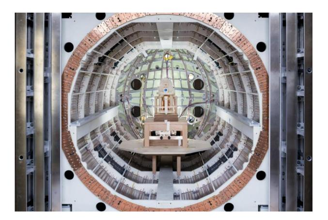
Inner three layers of the magnetic shield (also known as the insert), and the cylindrical layer with 780 copper rods. The cylindrical layer is used to generate a very uniform magnetic field, which is necessary for EDM experiments. Also shown are two measurement devices: A mercury magnetometer is placed between the wooden support structure, and a high precision pendulum device, which is used for the absolute alignment of conventional magnetic field probes,
